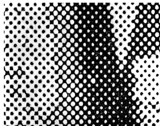
A section of a halftone letterpress print enlarged to show the dots. The effects of the paper roughness and the imperfections of inking & printing can also just be seen.
